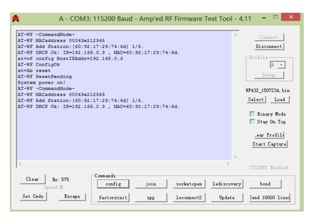
Step 6: Open socket on the Wi-Fi module side: At+wf socketopen
